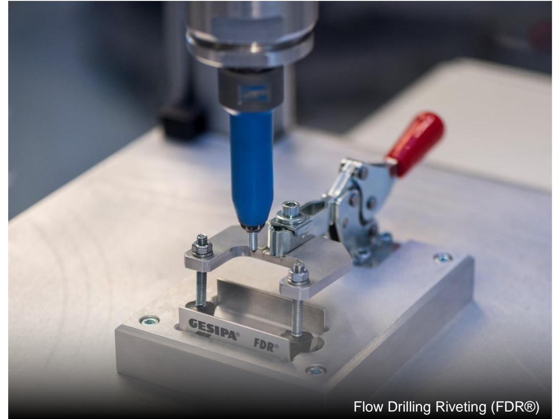
Flow Drilling Riveting (FDR®)
